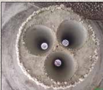
Exterior of the sensor is coated with dust, while self-cleaning properties keep the transducers clean and functional.
